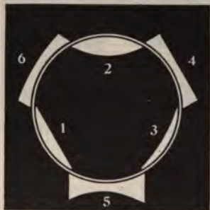
FIG. 147.—The Relation of the Surfaces of Lenses to Spheres. 1. Plano-convex; 2, biconvex; 3, convex meniscus; 4, plano-concave; 5, biconcave; 6, concave meniscus.
